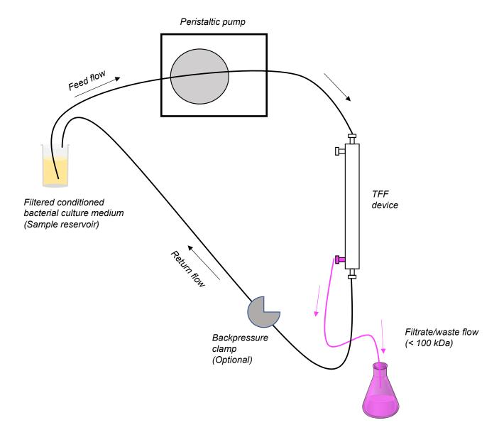
**Supplemental Figure S2: Tangential flow filtration (TFF) setup schematic.** The tubing with barb-hoses was connected to the TFF device as shown. Feed flow tubing begins submerged in the filtered conditioned culture medium vessel, continues through the peristaltic pump, and connects to the TFF device inlet port. The return flow begins at the TFF device outlet port and ends above the surface of the filtered conditioned culture medium. Optionally, a backpressure clamp
